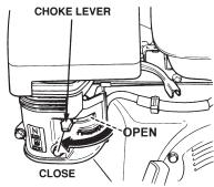
Figure 21. Choke Lever
